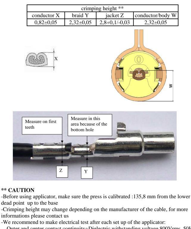
Outer and center contact continuity+Dielectric withstanding voltage 800Vrms, 50Hz Insulation resistance 1000 Mohms
